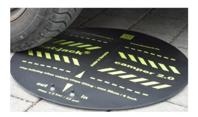
**3** Ensure centered tire position. Inflation valves must be accessible from outside.
